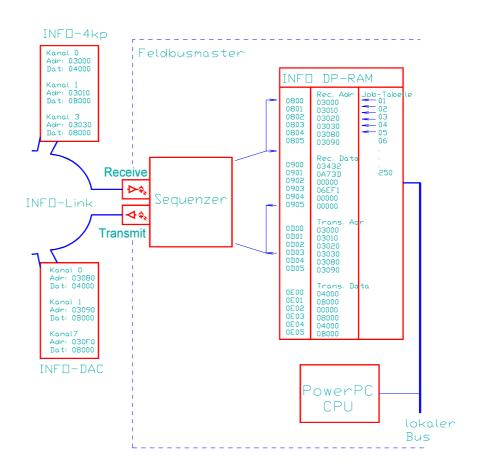
Functioning principle of the sequencer
