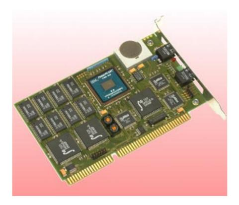
The INFO-PowerPC board is the field bus master via an INFO-Link. It is available as an PCI-bus or ISA-bus plug-in board and can be operated in any PC or industrial PC (IPC) with the INCO server. The heart of the master is the powerful RISC-CPU: PowerPC 603E, with 200 MHz clock rate. The real-time multitasking operating system of the master performs the entire control of the machine or plant. In other words, the master operates fully
