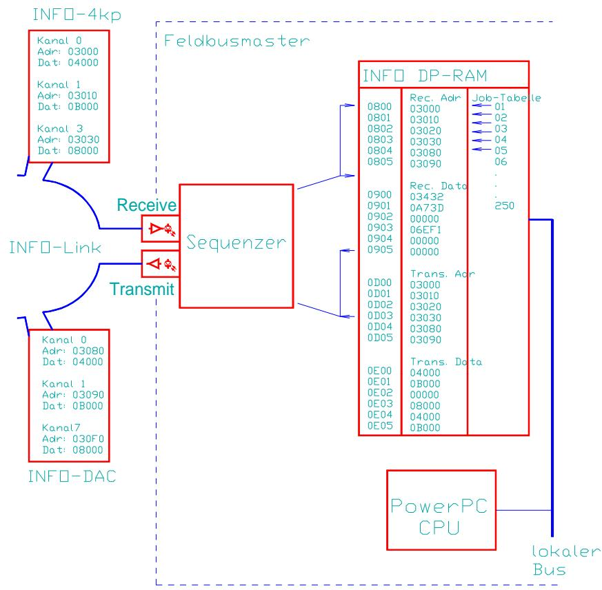
Functioning principle of the sequencer
