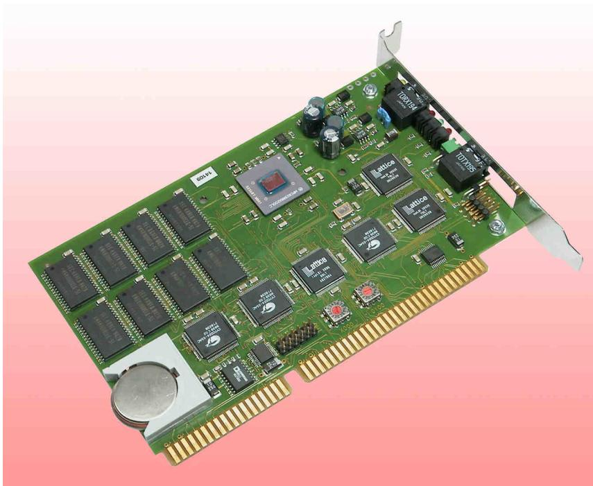
The INFO-PowerPC board is the field bus master via an INFO-Link. It is available as an PCI-bus or ISA-bus plug-in board and can be operated in any PC or industrial PC (IPC) with the INCO server. The heart of the master is the powerful RISC-CPU: PowerPC 603E, with 200 MHz clock rate. The real-time multitasking operating system of the master performs the entire control of the machine or plant. In other words, the master operates fully
