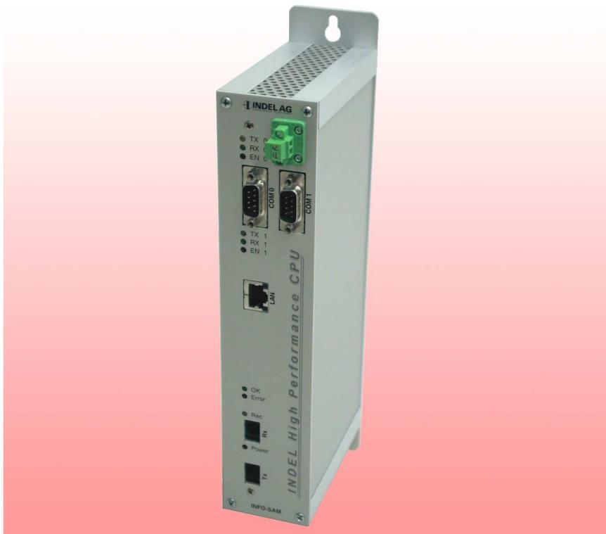
The INFO Stand Alone Master board is the field bus master of an INFO-Link. The board operates entirely autonomously and does not need any higher-ranking computer for operation. For visualisation and software updates, a 10 MBit Ethernet port and two RS232 interfaces are available. The real-time-capable multitasking operating system of the master per-
