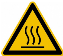
Figure 1: Warning: "Hot surface"
